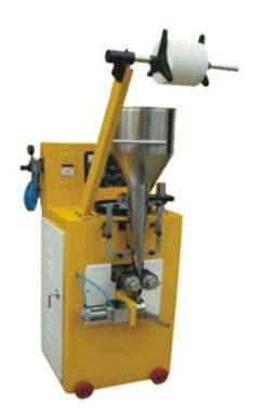
Use For :Tea, Pan Masala Etc, Products The Machine Requirment For Air – Compressor
