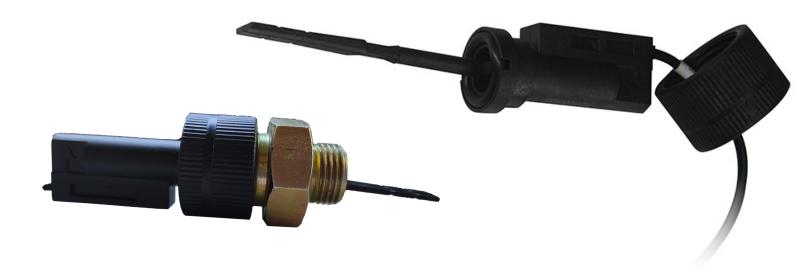
Flow switch consists of magnetic core, rotating impeller, external casing and dry reed pipe. Flow through the sensor activates the magnetic core to trigger switch action, with signal output.
