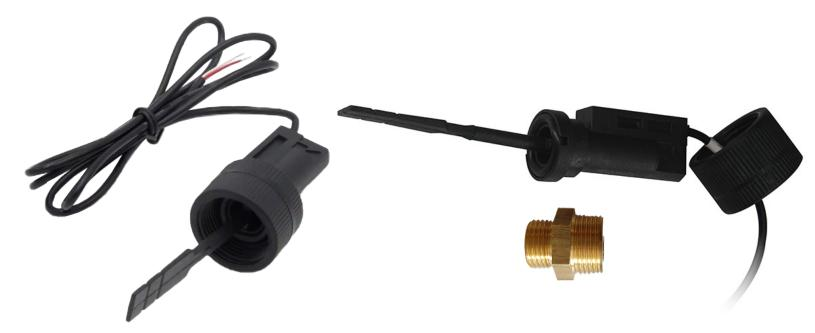
Flow switch consists of magnetic core, rotating impeller, external casing and dry reed pipe. Flow through the sensor activates the magnetic core to trigger switch action, with signal output.
