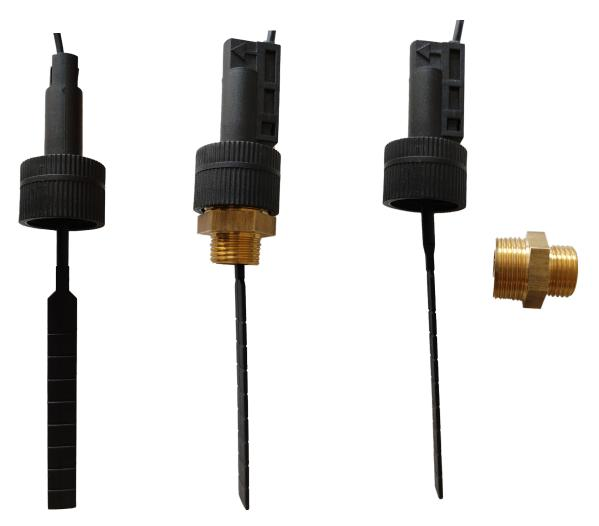
Our Long Paddle flow switch has speacial switch, used asspeacially for Big Diameter Pipes. Flow switch consists of magnetic core, rotating impeller, external casing and dry reed pipe. Flow through the sensor activates the magnetic core to trigger switch action, with signal output.
